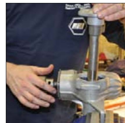
21. Next, grease the large teeth on the sector shaft and the new wormshaft, as well as the worm threads, and pack the case as full of grease as you can. Back off the adjuster screw at least 3 or 4 turns, and run a bead of RTV around the case opening, then drop in the sector shaft. Have the wormshaft in the center of it's range while doing this. The worm gear will need to be held upward with you finger so the sector gear will be able to slide in.
