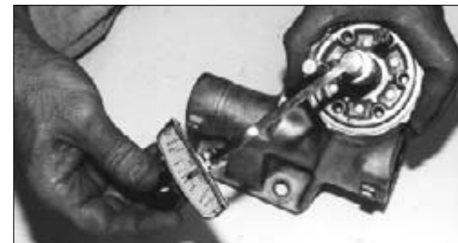
20. Tighten the adjuster so that the turning torque is at least 20-30 inch-lbs. A 11/16-inch, 12-point socket fits the splined shaft perfectly. Then turn the shaft lock-to-lock at least 3 or 4 times. Next, back off the adjuster, then tighten again until the turning torque is 1.2 to 4.5 in.-lbs. If the bearings are new, use the higher spec., otherwise, shoot for around 2.0 in.-lbs. Then reinstall the large locknut and tighten (with the punch).
