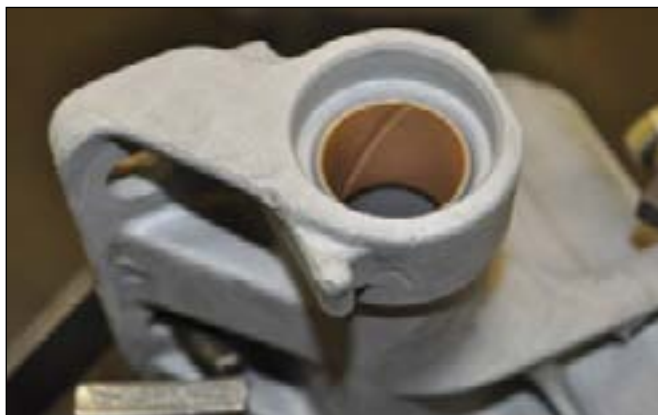
12. Six cylinder A-bodies had bushings on the sector shaft. They can be replaced with needles, but you can't do this yourself, since...
