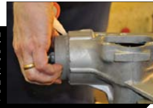
18. Although the case will be filled with grease (Dick recommends EP NLGI Grade 2), be sure to hand-lube the important areas before assembly. Wormshaft goes in first.
