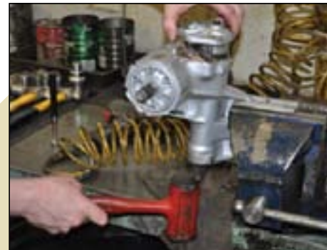
5. Disassembly begins by removing the sector gear cover (3 screws) and tapping the shaft out with a rubber or dead-blow plastic hammer, or block of wood and BFH.
