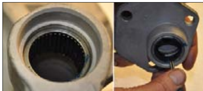
17. Here's the new sector needle bearings installed and lubed. Bearing lettering reads: "USA".
