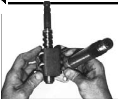
2. This hand-held mockup helps explain the principle of operation. The wormshaft (left) is connected to the steering column, the sector shaft (right) receives the pitman arm. Pretty simple, really.
