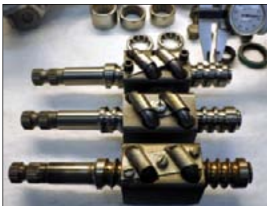
2. This hand-held mockup helps explain the principle of operation. The wormshaft (left) is connected to the steering column, the sector shaft (right) receives the pitman arm. Pretty simple, really.
