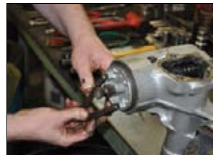
7. You'll need a pin spanner to remove the adjuster. You could rig up something from a scrap of steel and two screws.
