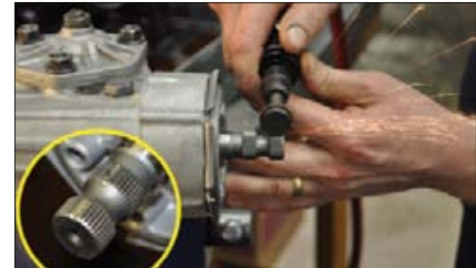
23. All that remains is cutting or grinding the master spline. This must be at 12 O'clock, with the gear in the exact center of its travel. This point should coincide with maximum turning-torque reading, you should also confirm that there close to the same number of turns (and fractions of a turn) in both directions, CW and CCW. You need to remove exactly one tooth. We used a die grinder, a Dremel tool with a super-small cutoff wheel would be mint. Put some tape over the seal while grinding to keep the chips away from the seal lip.
