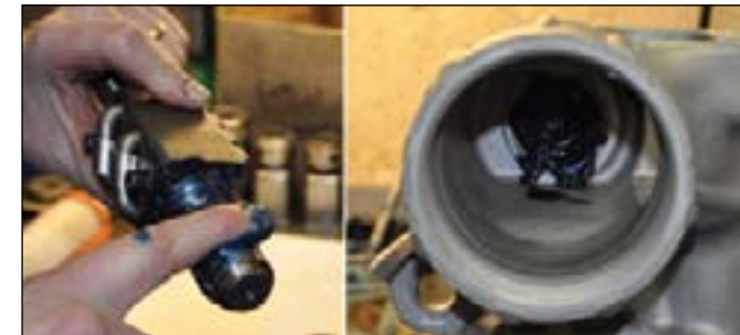
18. Although the case will be filled with grease (Dick recommends EP NLGI Grade 2), be sure to hand-lube the important areas before assembly. Wormshaft goes in first.
