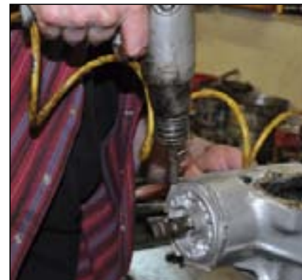
6. Unless you have a 3/2" inch socket or box wrench, you'll probably remove the wormshaft adjuster with a pin punch. This is okay as long as you're careful not to trash the delicate aluminum threads on the adjuster itself. A brass punch is good insurance.
