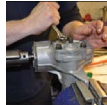
22. Torque the cover screws to 25 ft./lbs. - not inch-pounds! With the same torque wrench setup as photo 21, tighten the adjusting screw so that the torque reading as the wormshaft is moved though the center high-spot range is 7 in.-lbs. more than what you set in step 21. Then tighten the locknut.
